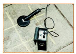
Elcometer P100 Imp Rebar Locator
